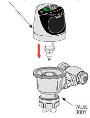
To facilitate installation, the 0-ring on the diaphragm assembly must be wet for easier insertion. NOTE: Sensor Lens must face directly forward. Rotating the Sensor to either side will decrease the Sensor's ability to detect a target.
