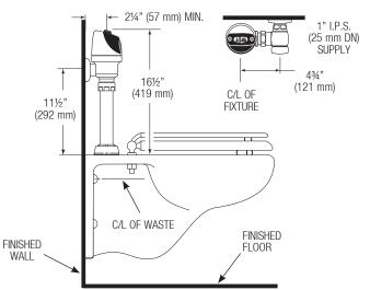
High Rough-in Water Closet Installation Models 8113, 8115 & 8116
